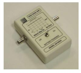
The SA1020 is a generally purpose, battery powered amplifier particularly suited to radiated emission measurement applications covering the range 9KHz – 1GHz.
