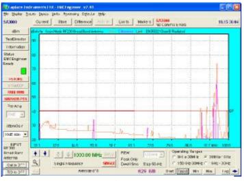
The difference trace is also invoked. This highlights the 50 and 70MHz peaks, and also shows a 90MHz emission plus some emissions in the 93 – 96MHz region. These latter are aligned with strong FM broadcast signals, and FM is by definition, a fluctuating signal.
