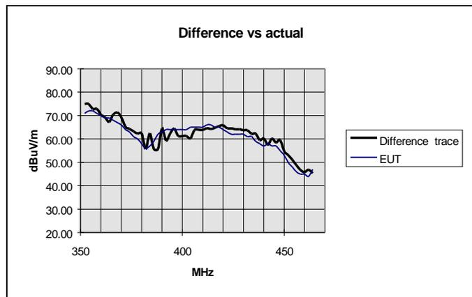
Subtracting two log values is the equivalent of dividing one by the other. So these values must be converted back to linear values first using the formula  $X(\text{lin}) = 10^{(X(\text{log})/20)}$ . Then the difference  $Z(\text{lin}) = X(\text{lin}) - Y(\text{lin})$ . Finally, Z is converted back to log (dB) values.  $Z_{\text{dBuV/m}} = 20\log(Z(\text{lin}))$ .
