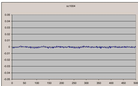
Plot sc1004 shows the ambient as output from the log periodic antenna with no sources switched on.
