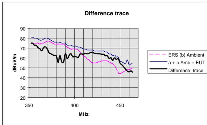
The third plot is a comparison of the estimated level and the actual level of emissions from the EUT. To calculate the signal which caused the field to rise from level XdBuV/m to level YdBuV/m we cannot simply subtract the two numbers to find the difference.
