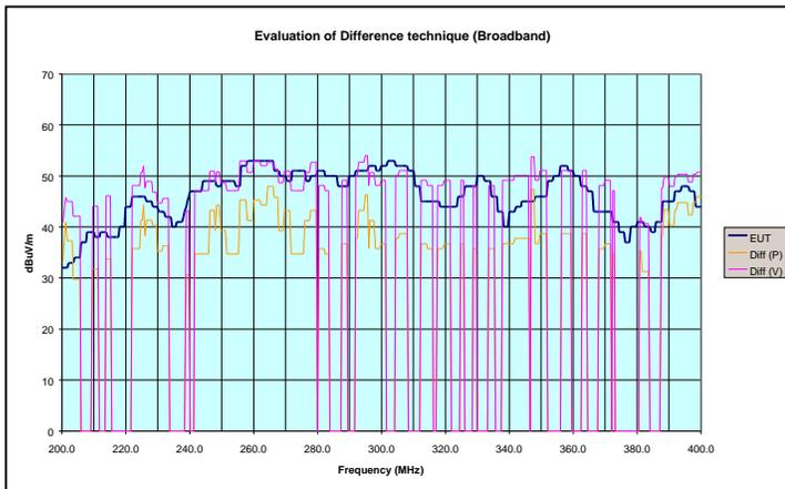
The final plot shows the actual EUT level and the difference trace as calculated for the narrowband experiment (Orange trace). The results show that the technique has failed to provide even a rough estimate of the levels from the EUT. Clearly the signals were not interacting together in the same way as the narrowband sources. In an attempt to improve the result, the difference was recalculated using a voltage base (V) rather
