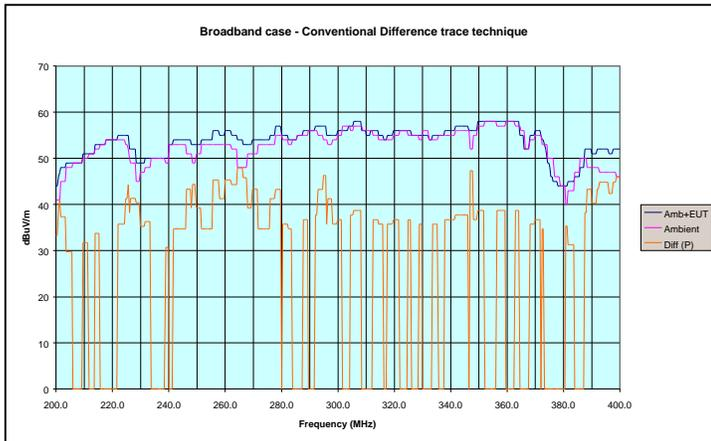
Then plots were taken with first one then both sources switched on. The plot shows the results. The difference trace includes intermittent excursions to minus infinity where the calculation attempts to find the log of zero! The cause of this little difficulty is at frequencies where the ambient result and the ambient + EUT result are the same (or negative).
