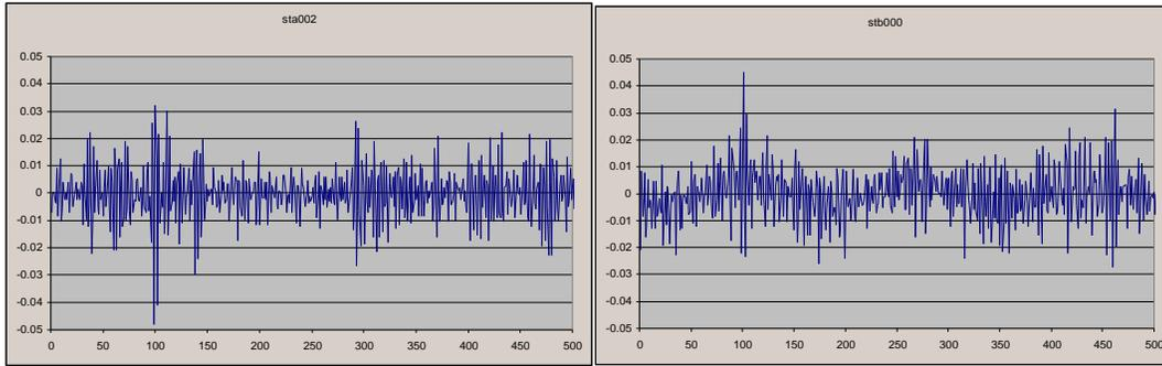
Plots sta002 and stb000 show the signal from the antenna with each source switched on independently. The impulsive nature of these sources is immediately evident. Fourier analysis shows that for a flat (ish) spectrum in the frequency domain, the time domain must have a transient nature. The signals are completely random in nature, as expected from noise sources.
